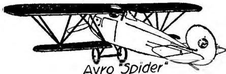
landing wires. And when it came to visibility that "one holer" in the top wing gave the pilot a look-see up and ahead. Even downward vision was good as the chord of the lower wing was very narrow.
